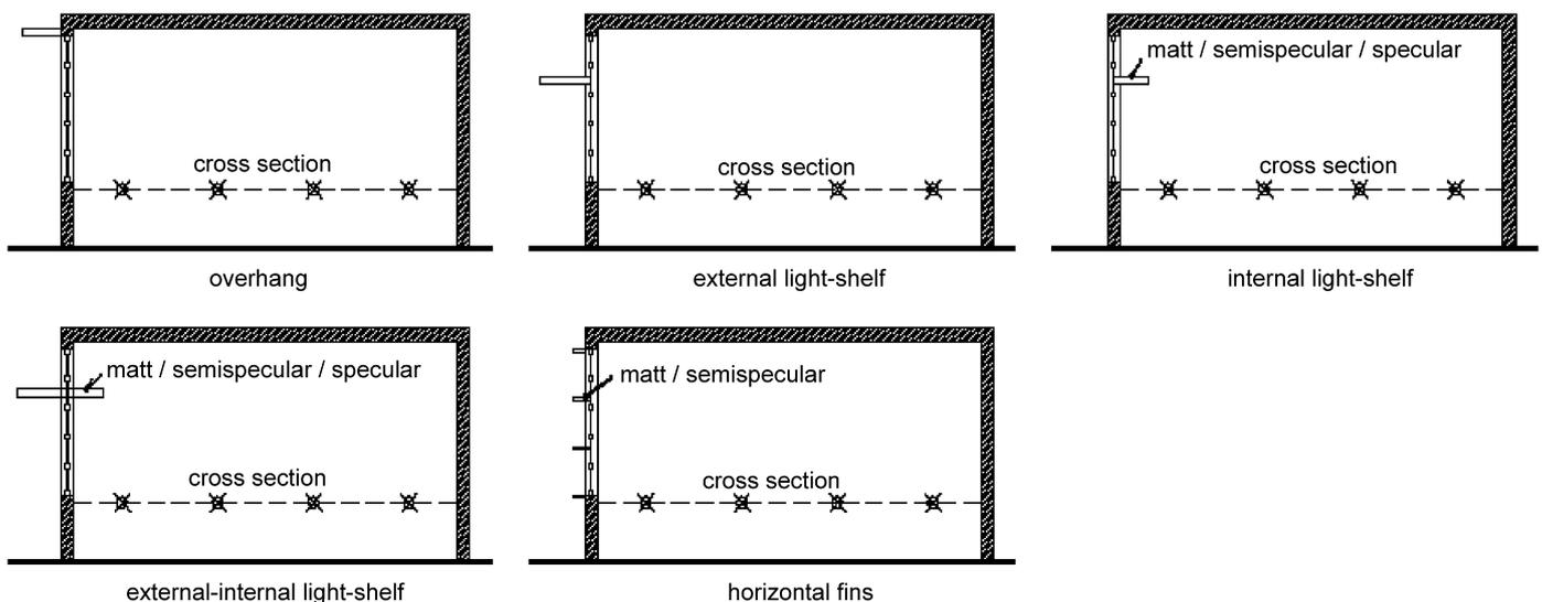
Fig. 3. Geometry and position of analysed shading systems.
