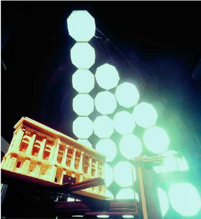
Fig. 1. The sky scanning simulator at the Daylighting Laboratory of the Politecnico di Torino.
