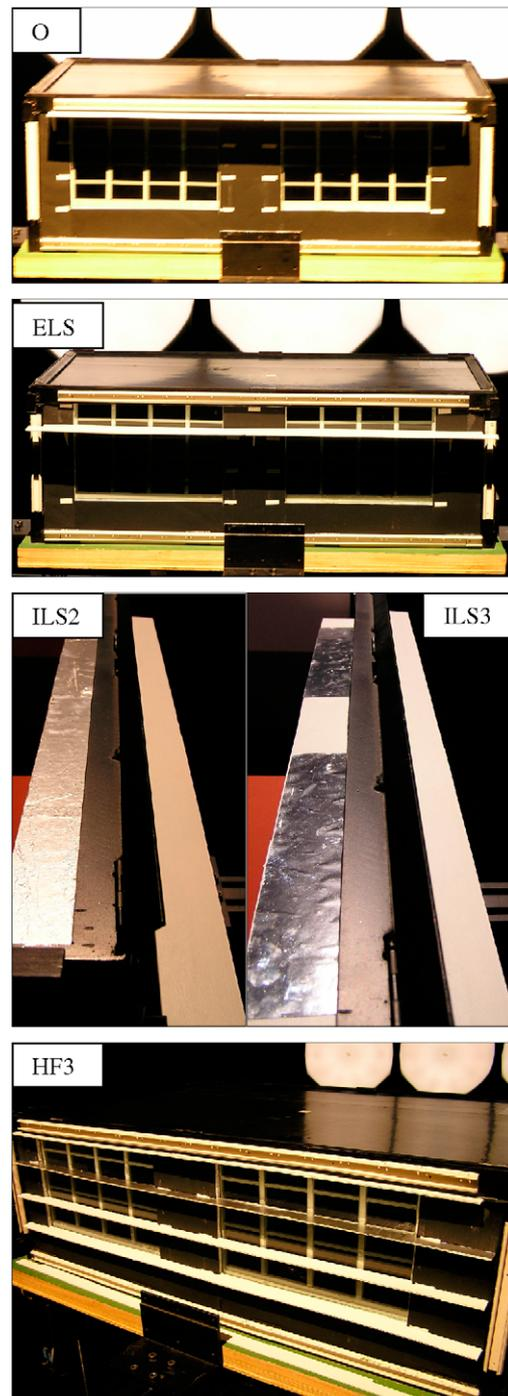
Fig. 2. Scale model reproducing a sample classroom equipped with different shading systems. From above to bottom: overhang, external light-shelf, external internal + light-shelf, horizontal fins. See Table 1 for legend.
