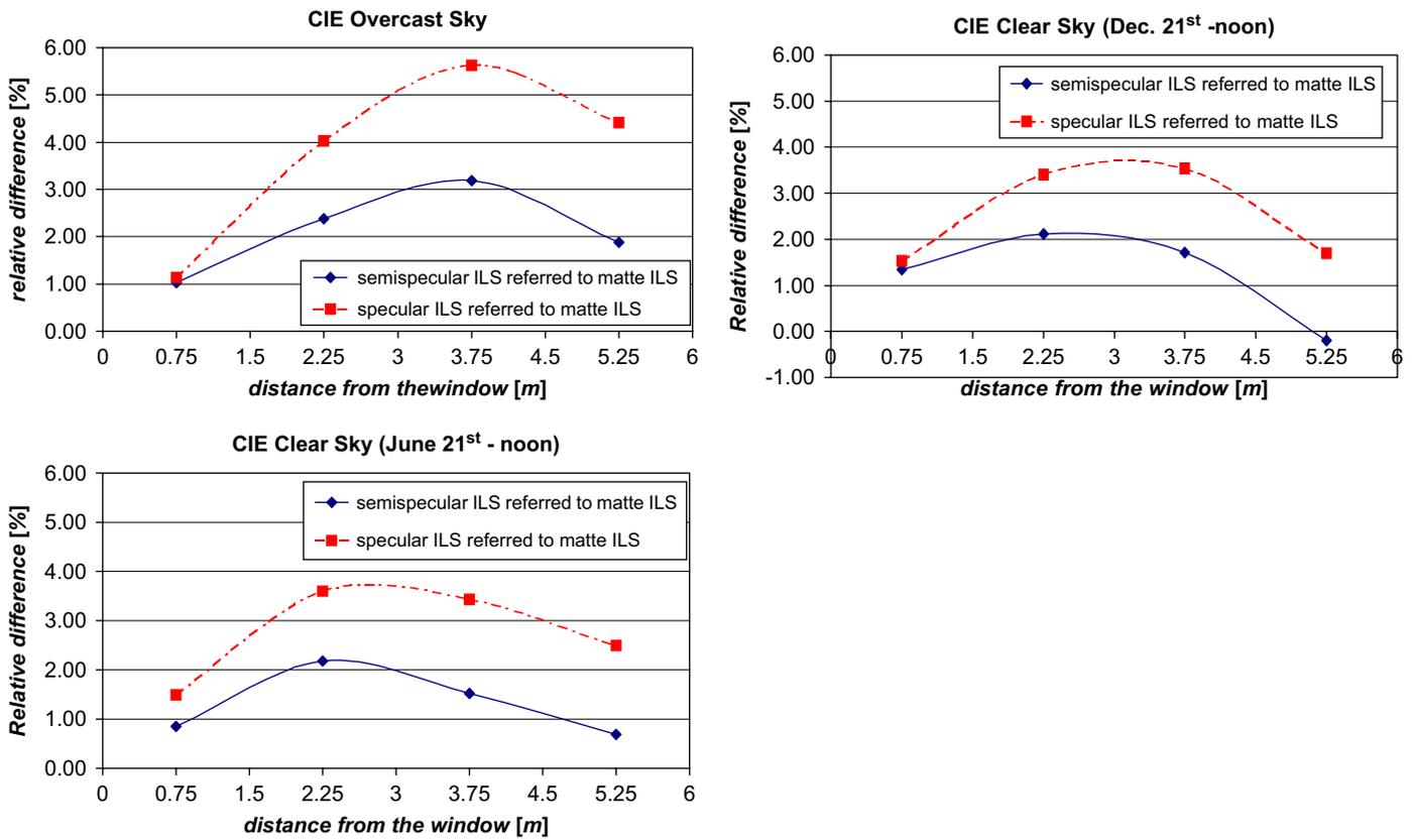
Fig. 8. Illuminance relative difference obtained with semispecular and specular finishing referred to matt finishing.
