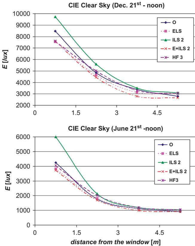
Fig. 5. Illuminance values measured along the cross section (reference condition: CIE Clear Sky).
