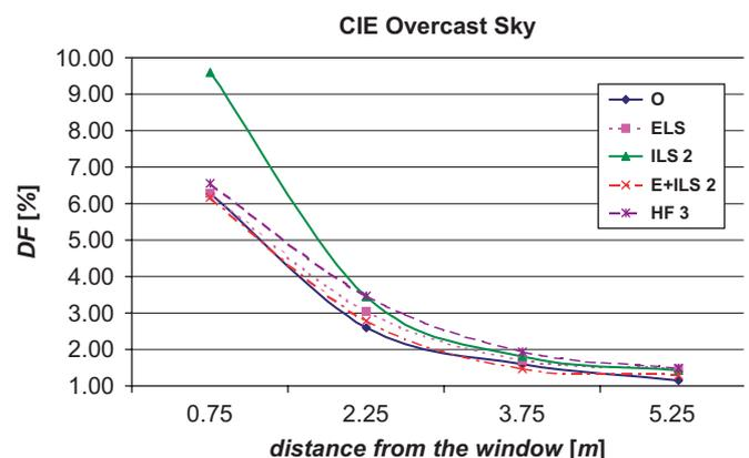
Fig. 4. Daylight factor values measured along a cross section (reference condition: CIE Overcast Sky).
