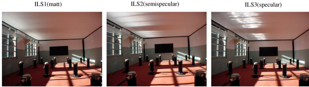
Fig. 7. Effect on light distribution on the ceiling produced by different finishing of the internal light-shelf.
