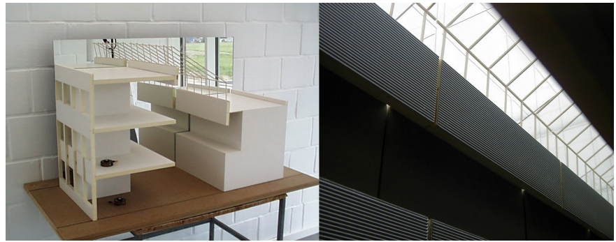
Figure 5: Example of mirror use for the modelling of symmetrical spaces (one mirror has been removed for taking the left picture).
