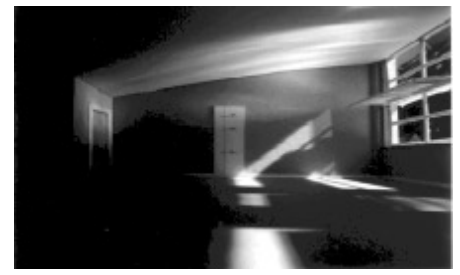
A student design exercise on an office, showing sunlight penetration in winter, in summer, and investigating the effect of a light shelf in summer.
