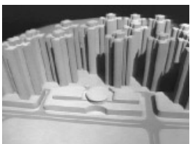
An investigation of a new housing estate in Hong Kong, checking shadowing and obstruction over the course of a day
