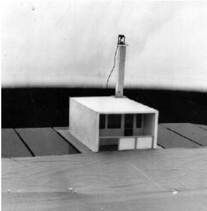
Fig. 5 Living room behind a loggia space in scale 1:10 under the ICA SAS artificial sky dome with exterior photocell
