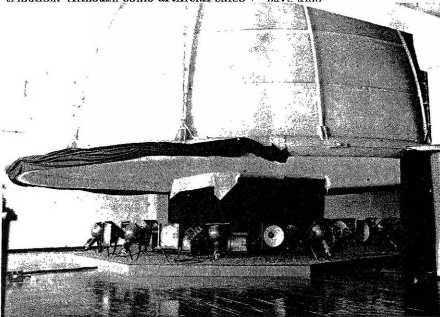
Fig. 1. New artificial sky at the Institute of Construction and Architecture, Bratislava.
