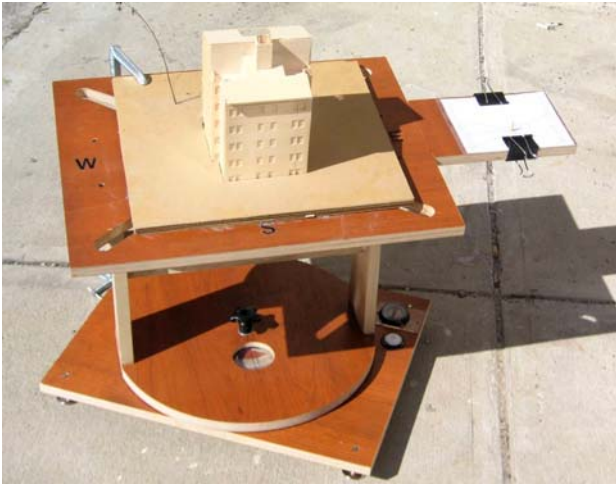
Fig.4: The portable heliodon, sunny operation.
