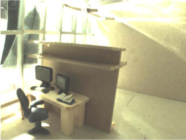
Fig. 11: An anidolic system can be a source of glare in direct light conditions.
